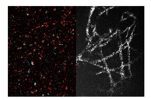
Thanks to a new technique that allows them to expand tissue 20-fold before imaging it, MIT researchers used a conventional light microscope to generate high-resolution images of synapses (left) and microtubules (right). In the image at left, presynaptic proteins are labeled in red, and postsynaptic proteins are labeled in blue. Each blue-red "sandwich" represents a synapse.
