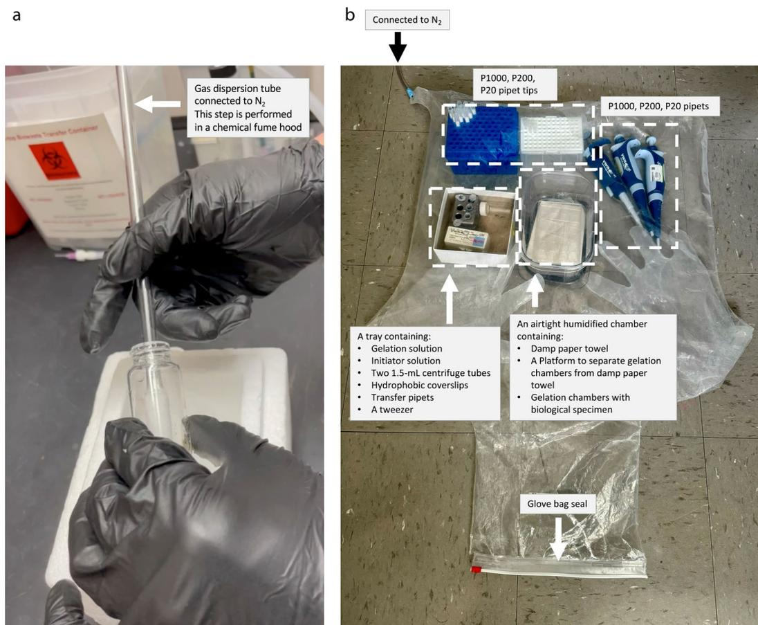
**Extended Data Fig. 2 | Oxygen-control setup of 20ExM.** (a) The gas dispersion tube is connected to a compressed nitrogen cylinder. With minimal  $N_2$  flow, the gas dispersion tube is placed within the gelation solution, with the sponge part fully wetted and generating bubbles. If the  $N_2$  flow is too strong, the gelation
