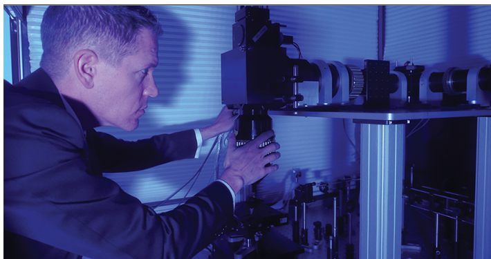
Figure 4. Smith's group designed an instrument called a dual independent enhanced scan engines for large field-of-view two-photon, or Diesel2p, which uses custom, large-scale optics to rapidly and simultaneously image neural activity over a large field-of-view (approximately 25 square millimeters). (Photo courtesy of Spencer LaVere Smith.)
