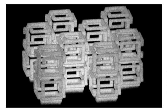
MIT engineers have devised a way to create 3-D nanoscale objects by patterning a larger structure with a laser and then shrinking it. This image shows a complex structure prior to shrinking.
