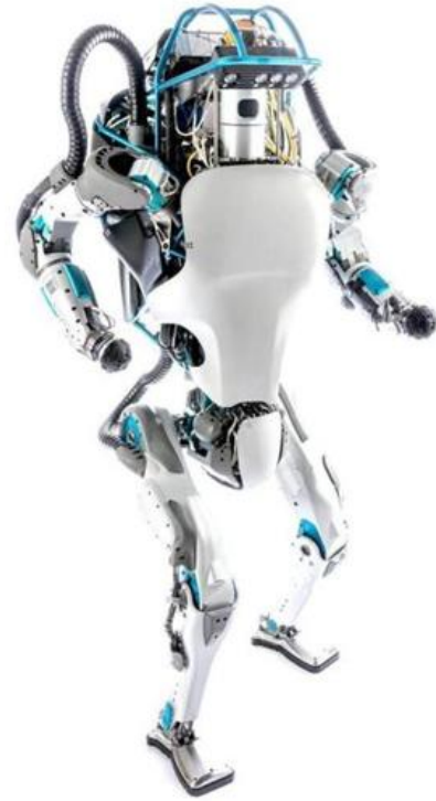
This next-generation Atlas is powered by a battery pack on its back.
