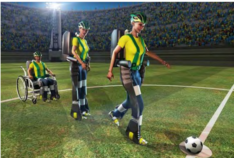
The design of an exoskeleton (external skeleton) that will allow paraplegics to walk again drew on basic neuroscience research. The exoskeleton uses computer algorithms to interpret the user's brain activity, which powers the exoskeleton forward. (Credit: Walk Again Project/virtualreality.duke.edu.)
