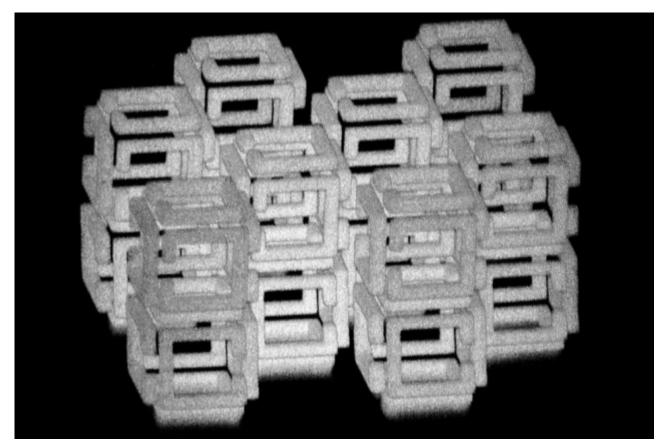
MIT engineers have devised a way to create 3-D nanoscale objects by patterning a larger structure with a laser and then shrinking it. This image shows a complex structure prior to shrinking. Image: Daniel Oran
