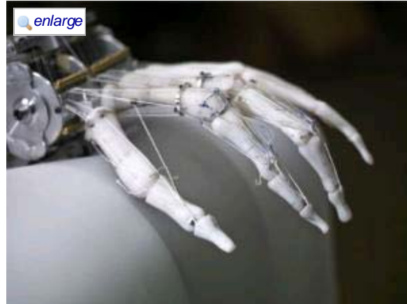
The Anatomically Correct Testbed Hand has three fully actuated fingers that have the same biomechanical structure as the human hand. This hand is used to understand the human hand's biomechanical structure and neural control strategies, and will serve as a prosthetic and surgical tool one day. (Credit: Ellen Garvens, University of Washington)
