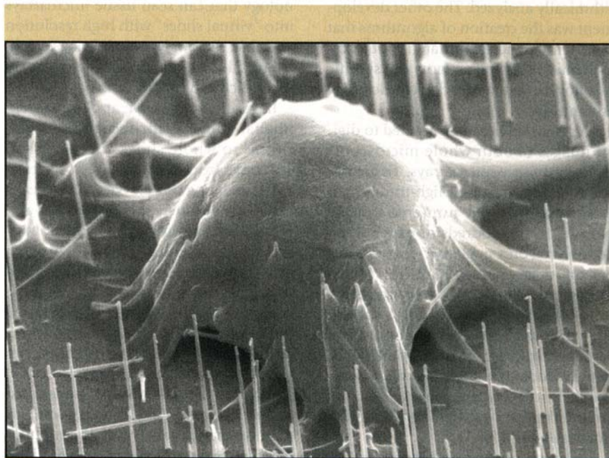
Scanning electron microscopy images demonstrate the penetration of individual mouse embryonic cells by 90-nm-diameter nanowires. No external force is necessary to facilitate penetration because of the small diameter and high aspect ratio of the nanowires.
