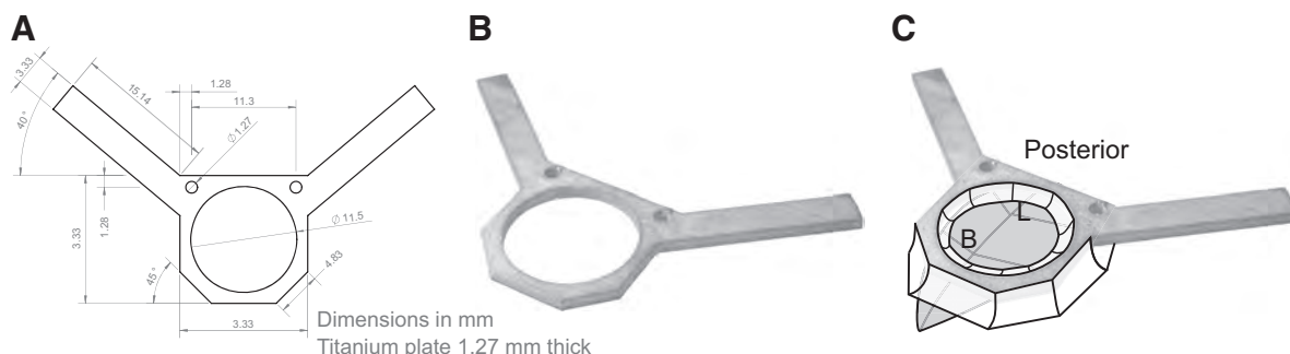
Fig. 2. Diagram of the head post (A and B) and dental cement application (C). In C, bregma and lambda are identified by B and L respectively.
