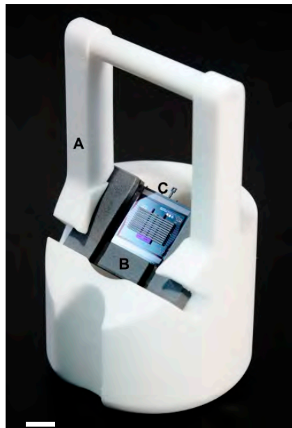
Figure 9. Teflon-based holder (A) for electroless plating. The darker insert (B) is specific to the probe (C) and holds the assembled probe at a 45-degree angle, to facilitate the removal of evolving gas from the plating sites to avoid gas getting trapped under a horizontal surface. The insert (B) can also be used to hold the probe during mechanical assembly steps (see section). The scale bar is 1 cm.
