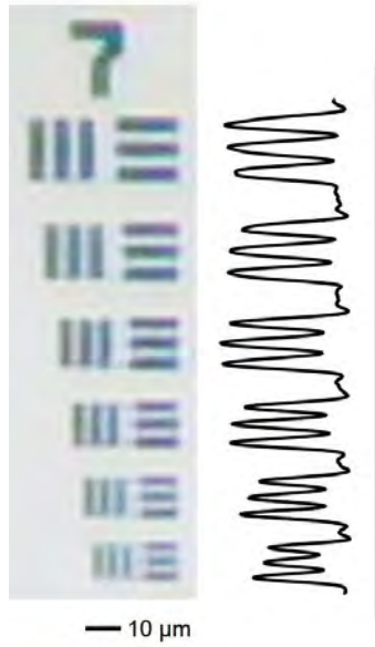
Supplementary Figure 1: Resolution determination of mini-microscope. Mini-microscope image of Group 7 resolution target and line profiles showing clear separation of the peaks between adjacent lines. The thinnest line width at the bottom is 2.19 μm.
